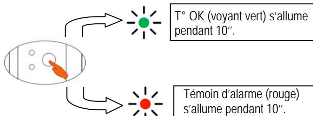
The action is recorded and will appear on the curve when you process the data with your software Sirius.
