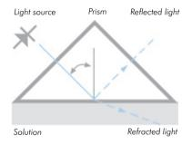
Depending on the angle, some rays are totally reflected. And, some rays are only partially reflected, most of the light is refracted into the process solution.
