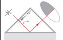
A digital CCD-camera detects the optical image and the shadow line. The camera transforms the optical image point-by-point to an electrical signal. The exact shadow line position is located and the refractive index  $n_{\rm D}$  is determined.
