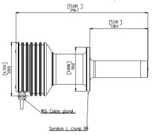
Sensor PR-23-GP with ANSI/DIN/JIS flange
