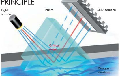
The light source sends light against the interface between the prism and the process solution, where the rays meet the surface at different angles.
