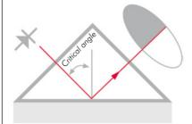
A digital CCD-camera detects the optical image and the shadow line. The camera transforms the optical image point-by-point to an electrical signal. The exact shadow line position is located and converted to a reading in refractive index.
